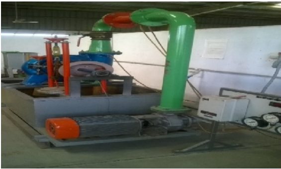
Fig. 4. Shows experimental setup of water pump with Francis turbine.
